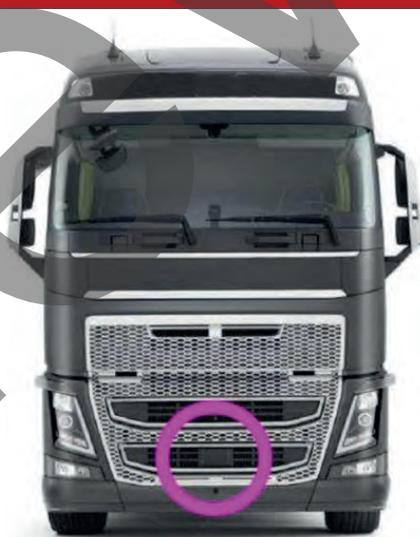
Figura 56: Radar position
