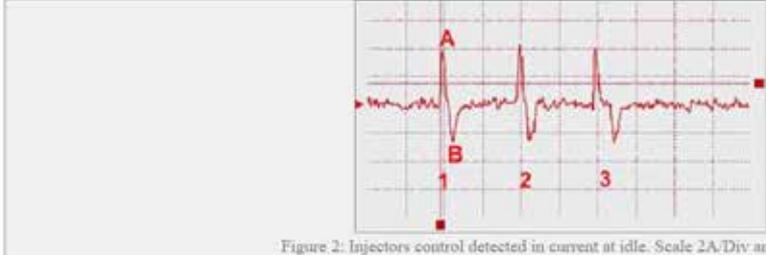
Figure 2: Injectors control detected in current at idle. Scale 2A/Div and 1ms/div
